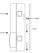
3. Once the DAI unit is mounted to the wall, the telephone connections can be made. Using four conductor modular cable with RJ-12 plugs, run a swapped cable from the Station In to a station jack on the control unit. Run two other cables from the Station A and B Out jacks to two separate analog telephone devices (*see diagram below*).
